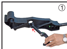
1.SUP KICK LEG BOTTOM INTO THE HOLE OF THE AXLE.
