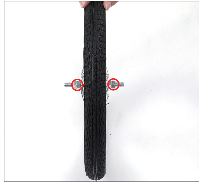
4-Tighten the axle using the nuts (2 on each side).
