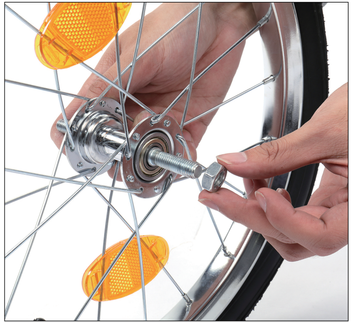
4-Tighten the axle using the nuts (2 on each side).
